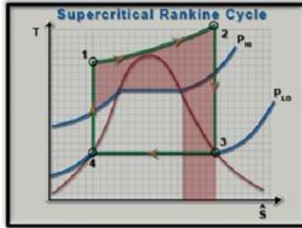
Figure 5 : T-S Diagram of Supercritical Rankine Cycle
