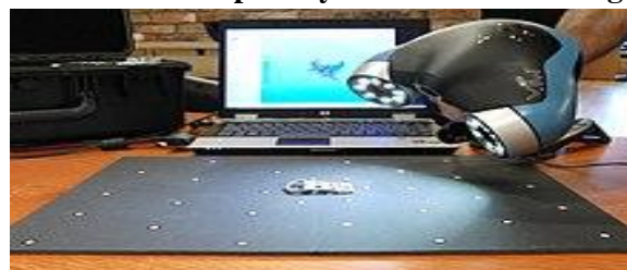
Figure 16 Making a 3D-model of a Viking belt buckle using a hand held VIU scan 3D laser scanner.
